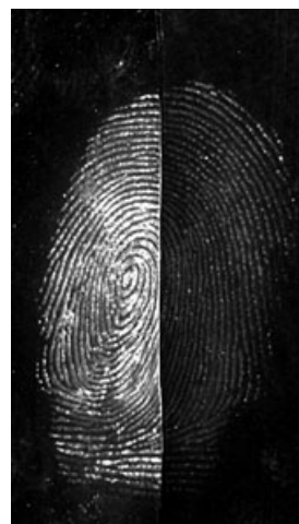
FIG. 11—Cyanoacrylate-developed fingerprint on a zip-lock bag stained with (left) rhodamine 6G (luminescence mode; excitation 505 nm, barrier band-pass filter 610 nm) and (right) styryl 11 (luminescence mode; excitation 590 nm, barrier band-pass filter 750 nm).
