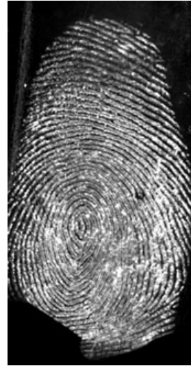
FIG. 15—Cyanoacrylate-developed fingerprint on glossy cardboard stained with STaR 11 (luminescence mode; excitation 530 nm, barrier band-pass filter 750 nm).
