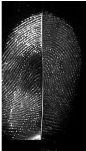
FIG. 13—Cyanoacrylate-developed fingerprint on a zip-lock bag stained with (left) rhodamine 6G (luminescence mode; excitation 505 nm, barrier band-pass filter 610 nm) and (right) STaR 11 (luminescence mode; excitation 530 nm, barrier band-pass filter 750 nm).
