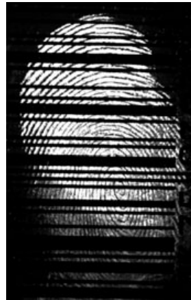
FIG. 16—Cyanoacrylate-developed fingerprint on a barcode on glossy cardboard stained with STaR 11 (luminescence mode excitation 505 nm, barrier band-pass filter 610 nm).
