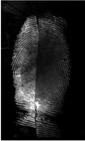
FIG. 12—Cyanoacrylate-developed fingerprint on a plastic bag stained with (left) rhodamine 6G (luminescence mode; excitation 505 nm, barrier band-pass filter 610 nm) and (right) STaR 11 (luminescence mode; excitation 530 nm, barrier band-pass filter 750 nm).
